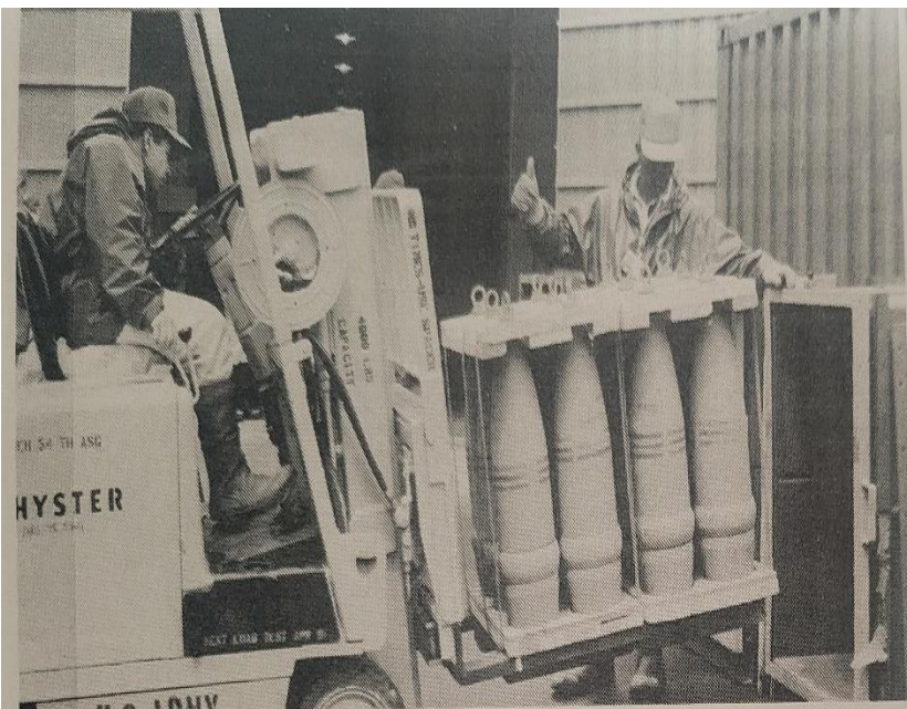
A forklift driver from the 59th Ordnance Brigade loads a pallet of chemical munitions into a vapor-proof Secondary Steel Container (SSC). Ground guides are always used to ensure safe loading of the projectiles. (Photo by SPCLJ. Teisel)
